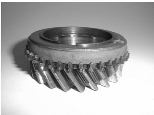
Links: Gangrad 901 / Rechts: Synchronring G50 Getriebe
